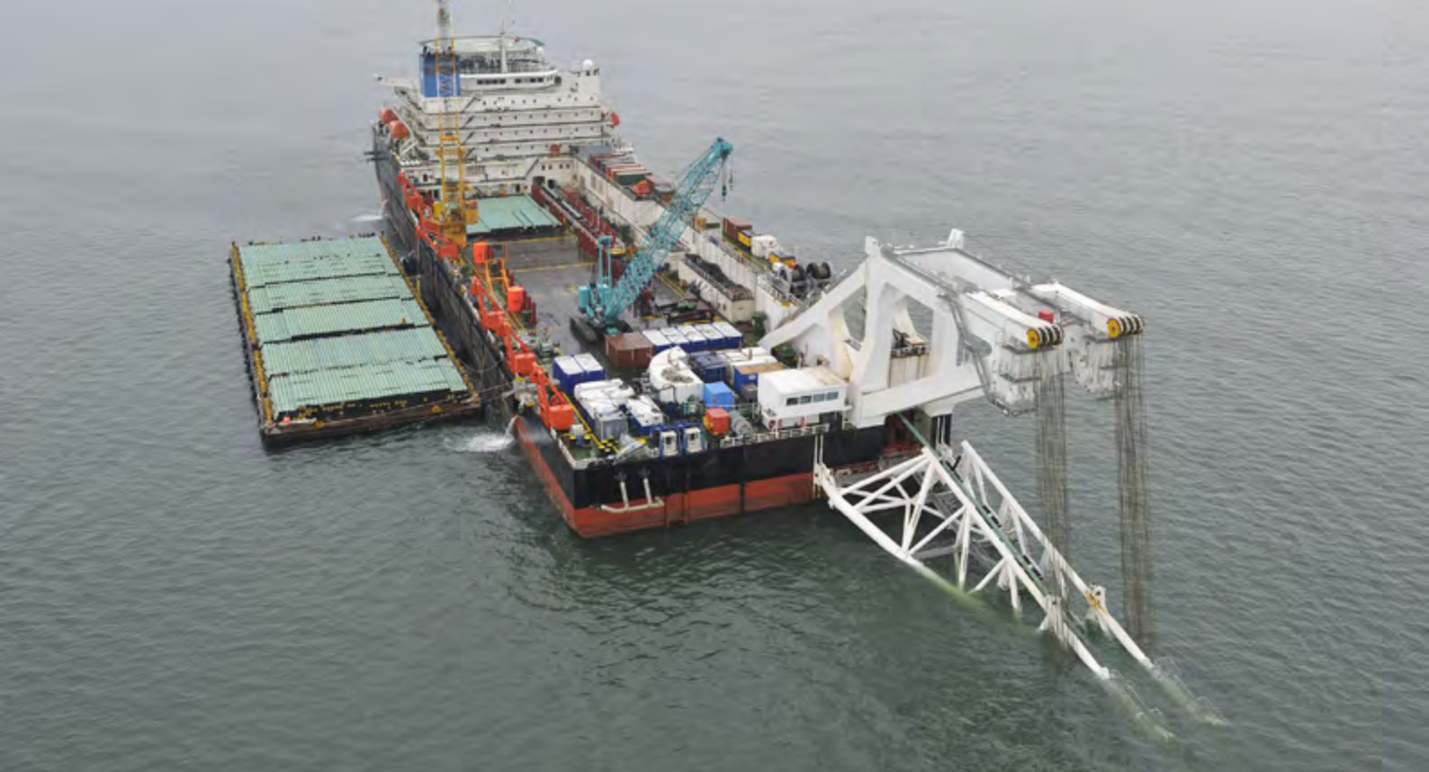
Pipe laying barge. ©Shutterstock_Alexey Alexandrov
